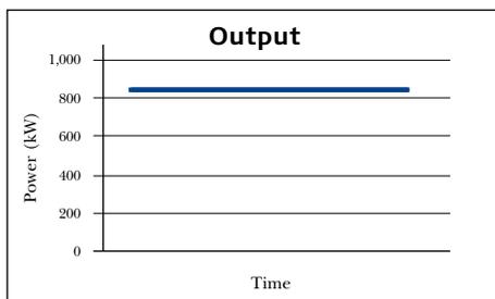
*OptiSpeed® allows the rotor speed to vary within a range of approximately 60 per cent in relation to nominal rpm. Thus with OptiSpeed®, the rotor speed can vary by as much as 30 per cent above and below synchronous speed. This minimises both unwanted fluctuations in the output to the grid supply and the loads on the vital parts of the construction.*
